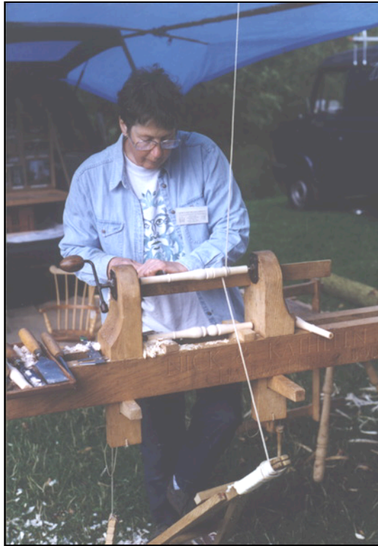
Fig. 1 - Pole lathe in use at Hatfield Forest Wood Fair - 5th September 1998
