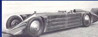
Henry Seagrave's Golden Arrow set new land speed record of 231 mph at Daytona Beach in 1929 powered by a Napier Lion engine
